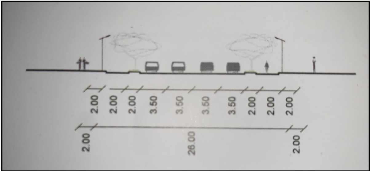
Figure 6 26-meter road for expansion area.
